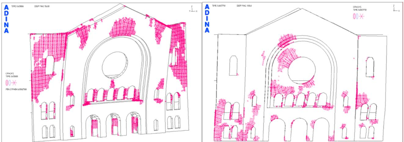
Figure 6 Deflected shape and cracking pattern of south wall due to out-of-plane (50X), and in-plane (100X) loading
