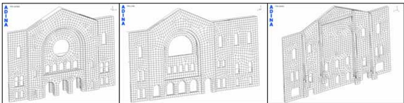
Figure 2 ADINA meshes for the south, west and north walls, respectively.
